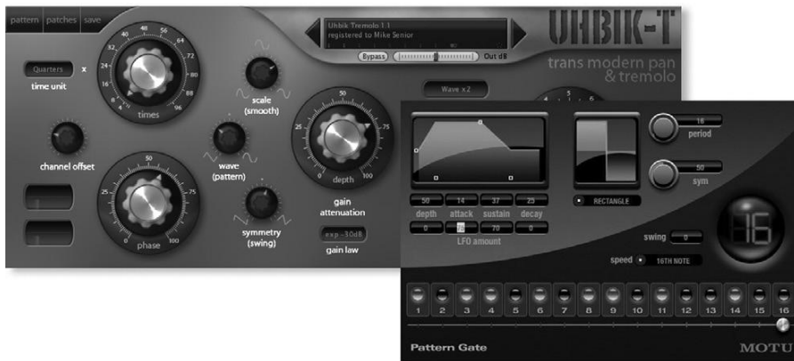
FIGURE 10.4 Programmable tremolo units (such as U-he's Uhbik-T, left) and tempo-synchronizable gates (such as MOTU's Pattern Gate, right) offer time-based balancing options that extend beyond the capabilities of normal level-based dynamics processors.
