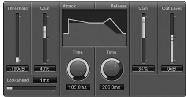
FIGURE 10.2 Logic’s Envelope Shaper plug-in is an example of a threshold-dependent transient processor.
