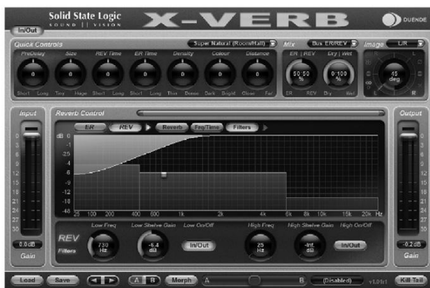
FIGURE 16.6 It's common to reduce the amount of low-end content in your reverb return (as shown in SSL's X-Verb here) to keep the low frequencies of your mix clear sounding.
